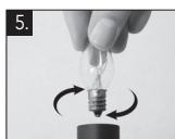
Take the new bulb, insert in the holder and twist it in the clockwise until it stops twisting further.
